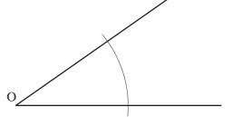
Then draw two further arcs of equal radius, using the points where the arc intersects the lines as the centres.
